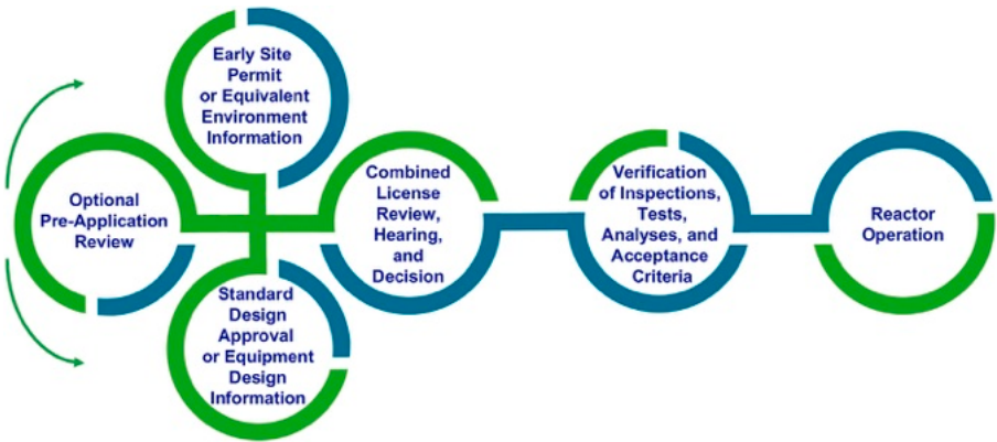
FIGURE 9 Flow chart of US NRC 10 CFR part 52 licensing process.
