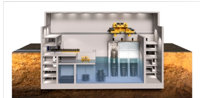
FIGURE 3 NuScale reactor building cutaway.
